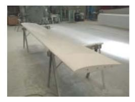
specially manufactured for exclusive catamaran, these centreboards are manufactured from carbon and glass fibres and epoxy resin.
